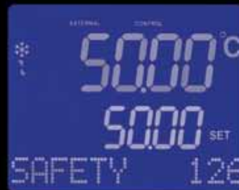
Class III safety features plus user-settable over-temperature safety and adjustable high and low temperature limits provide exceptional process and equipment protection.
